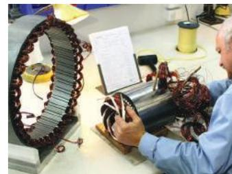
Bobinage de stator.
